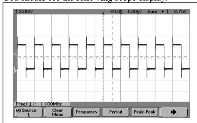
Figure 3 Master oscillator signal.
