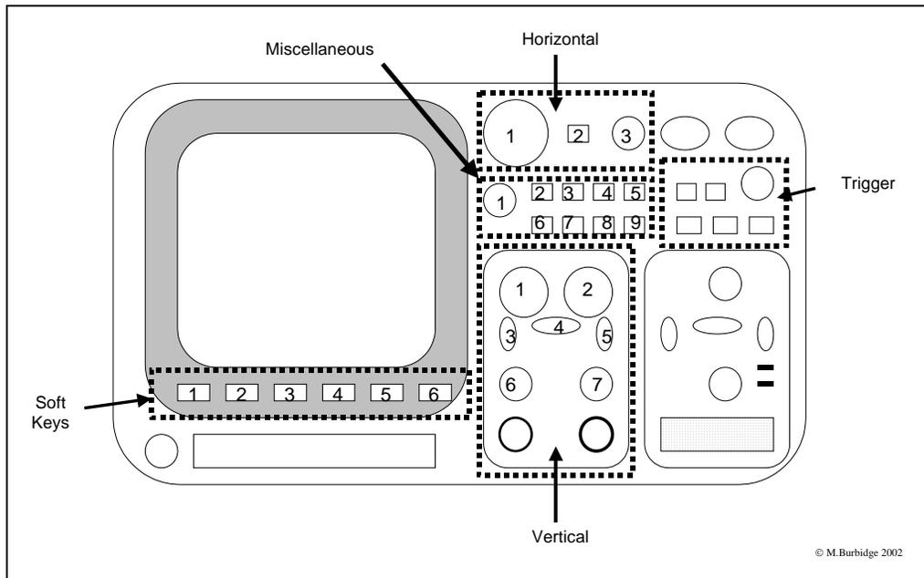
**Figure 2** Oscilloscope front controls
