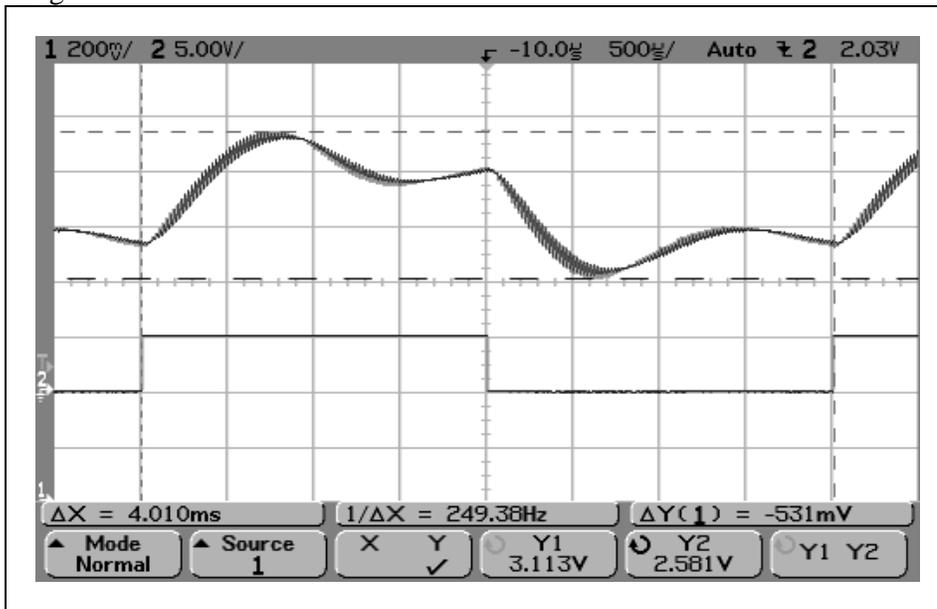
**Figure 5PII step response display.**
